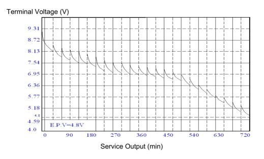
Figure 2: GL6F22A DISCHARGE CURVE
